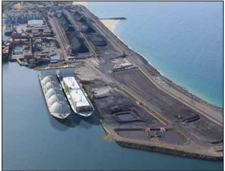
*A depiction of an LNG tanker alongside a floating storage and regasification unit (FSRU) at the gas import terminal proposed for Port Kembla, NSW.*
